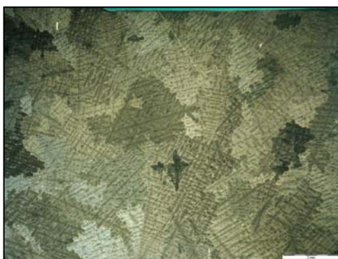
Fig. 1a Macrostructure of the lock turbine blades with dendritic segregation
