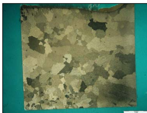
Fig. 1b Macrostructure of the surface turbine blades with dendritic segregation
