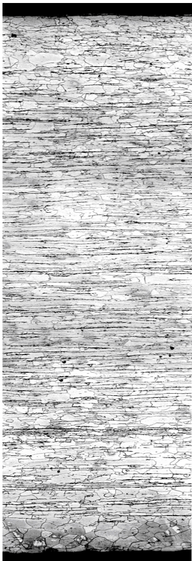
Fig.1 Microstructure of grain oriented silicon steel (Cu content of 0,44%) after hot rolled strip
