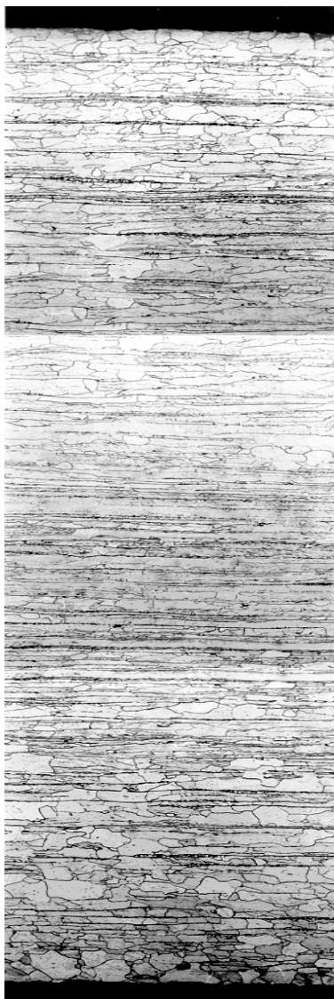
Fig.2 Microstructure of grain oriented silicon steel (Cu content of 0,03%) after hot rolled strip
