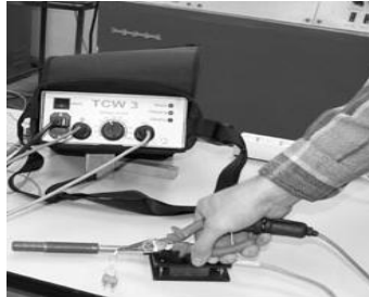
Fig.6 Welding of thermocouple
