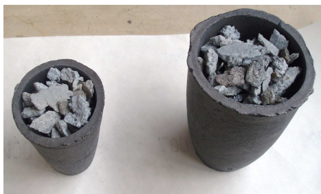
Fig.1 Bottom dross before refining
